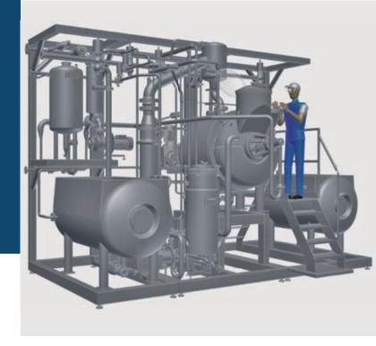
The JamMod600 cooking module thaws frozen fruit in a defrosting container. The fruit is then cooked in a process vessel after mixing in sugar, pectin and other additives. Once the cooking and thickening processes are complete, filling continues from the buffer container. The equipment is designed to ensure minimum product losses, short cooking and cleaning times, to maintain the lumpiness of the product as well as the natural colours and taste of the raw fruit.
