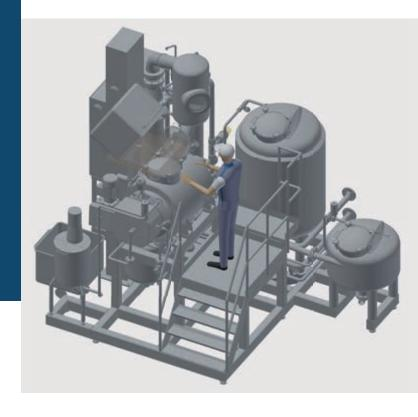
The JamMod250 cooking module enables the cooking of fruit mixed with sugar, pectin and other additives, as well as the subsequent thickening under vacuum in a single process vessel. The equipment is designed to ensure minimum product losses, short cooking and cleaning times, to maintain the lumpiness of the product as well as the natural colours and taste of the raw fruit.
