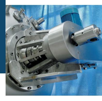
KASAG's bearing and mechanical seal (GLRD) offers advantages compared to other solutions in terms of all operating and wear criteria. The design of these seals enables extended life spans and simple maintenance along with low operating cost.
